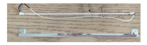
Step 5: Get your Monitech LED Backlight Replacement (MB084SN03V1). Take the tape cover off the Monitech LCD backlight. Stick the LED Strip in the Backlight housing.
