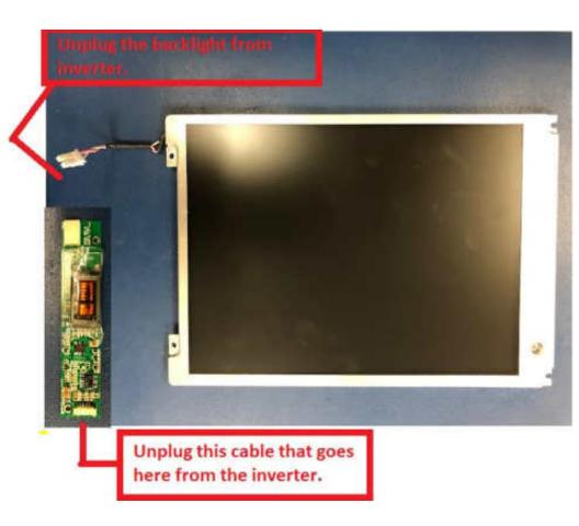
Step 4: Unscrew the backlight housing from the LCD. Take out the CCFL Backlight from the metal housing.
