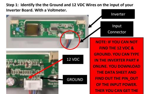
Step 2: Now that you have idenfitied the 12 VDC & GROUND you can take the wires out of its connector. Then connect the ground of the invertor input to our black coming out of our board. Then connect the 12 VDC of the invertor input to our red coming out of our board. Use the white dual clip black connector to connect the wires together.
