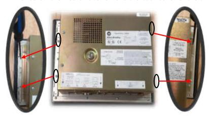
• Disconnect the CCFLS bulbs cables and then the power cable of the inverter.
