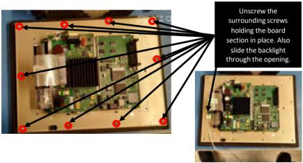
Unplug the old backlight connector. Slide the old backlight out of the LCD panel, you may need a small flat head screwdriver to unlock the backlight holder.
