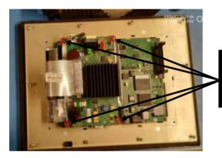
Unscrew the 4 screws holding the power supply board and remove it.
