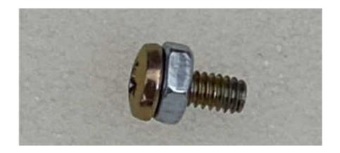
Add nut onto each screw as a spacer and install the new LED backlight and re-install the screws
