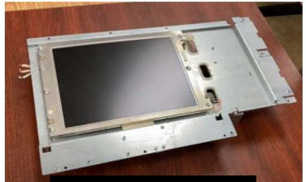
Remove the LCD Panel and remove the 4 screws for the backlight
