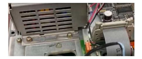
Remove this red wire. It is the power for the old CCLF backlights. It is not required and MUST BE REMOVED!
