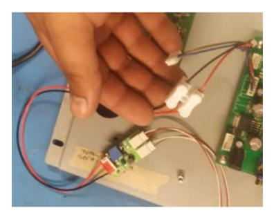
Step #6) Now mount our inverter board by using the double sided tape or using the the M3 Nylon hardware provided to you in the package. Use the zip ties to secure any loose wires.
