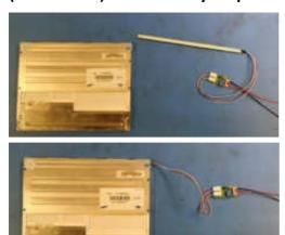
Step #4) Identify the the Ground and 12 VDC Wires on the input of your Inverter Board. With a Voltmeter.
