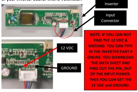
Step #5) Now that you have idenfitied the 12 VDC & GROUND you can take the wires out of its connector. Then connect the ground of the invertor input to our black coming out of our board. Then connect the 12 VDC of the invertor input to our red coming out of our board. Use the white dual clip connector to connect the wires together.
