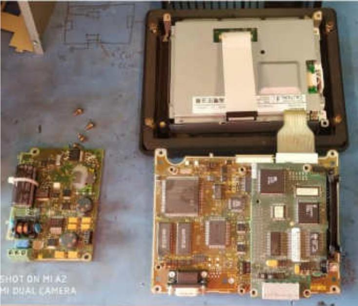
**UNSCREW THE LCD OUT OF THE BEZEL.**
