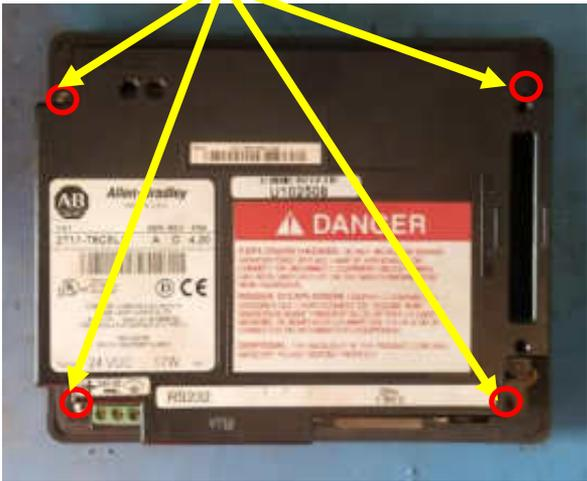
UNSCREW THE SCREWS HOLDING THE POWER SUPPLY IN PLACE. REMOVE THE POWER SUPPLY.
