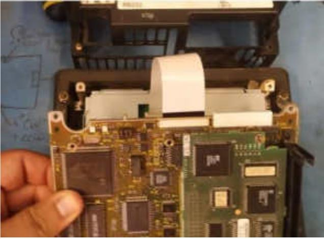
**SCREW IN THE BOARD INTO THE FRAME.**
