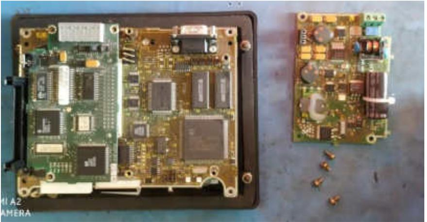
UNSCREW THE SCREWS HOLDING THE BOARDS IN PLACE.
