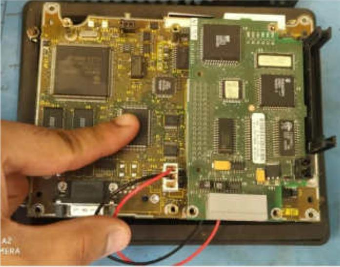
PLACE THE POWER SUPPLY BOARD BACK ONTO THE MAIN BOARD
