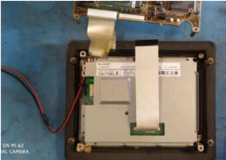
**PLUG IN THE LCD RIBBON CABLE INTO THE BOARD.**
