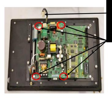
Unplug power connector. Remove power supply (top board—4 screws and 4 wires).
