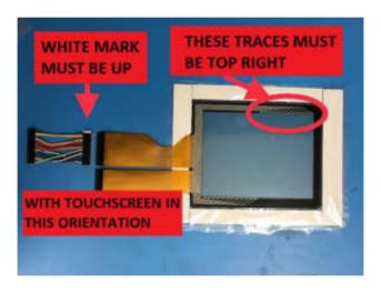
Step #4) Connect the multi colored cable to the connector on the replacement touchscreen.
