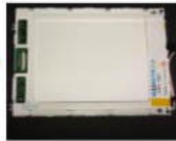
LCD PANEL LMG5320XUFC for the Fanuc A02B-0200-C081 & A02B-0210-C040 (LMG5320XUFC)
