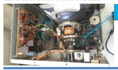
Logic board Unplug the video & power cable. For Xycom 2005, there is 2 types of connector we have seen in the CRT.
