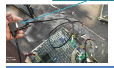
Step 11) Test the monitor before screwing the HMI back in. Plug power back in and screw the ground back in. Turn on power. If good put screws in to fasten the HMI. Use the user guide to Adjust Image.
