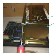
Unscrew the 4 screws to remove the cover of the CRT.
