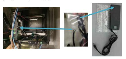
**Step #16)** Close the computer section and mount it in with screws. Connect the Video cable into the Monitech monitor. Plug in the power jack into the Monitech Monitor.
