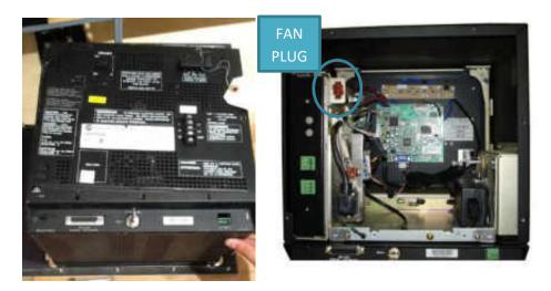
**Step #5)** Remove the screws and nuts, that is holding the black cover on the bezel. Keep all fasteners for re installation.
