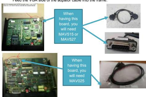
**Step #15)** If you are using MAV527 or MAV515. You must use the MAP351 power apator cable connect as shown on your panelview power supply. Then connect it to MAP307.
