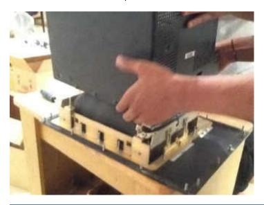
**Step #6)** Remove high voltage from the CRT by placing a screwdriver underneath the rubber of the anode lead and the other end touch metal, with another screwdriver put the tip onto metal and cross it with the first screwdriver. Then remove the anode lead by pushing one contact in so that it.
