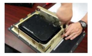
**Step #12)** Place the Black cover back on with screws prevousily taken off. Then mount the power supply part back in.
