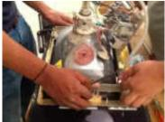
**Step #8)** Unscrew the nuts holding the gold CRT frame in place. Take it off the front bezel. Keep all fasteners for re installation.
