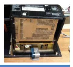
**Step #4)** Remove the back cover, by unscrewing the surrounding fasteners that mount the cover in place. Disconnect the single ground or if you have a fan, disconnect the fan plug. Keep all fasteners for re installation.
