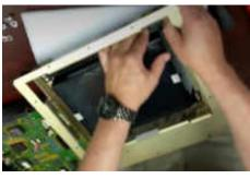
**Step #11)** Now take the Monitor that is attached to the old CRT frame and attach to the front frame with the fasteners prevously take off. Make sure the touchscreen cable does through the hole.
