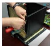
**Step #13)** Place the computer section back in. Connect the power supply connector and the touchscreen connectors to the board.
