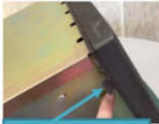
THESE HINGES ARE THE HINGES KEEPING THE HMI UNIT IN PLACE
