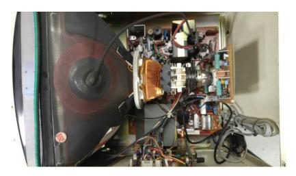
**Step #4)** Take Anode Lead off the CRT with pliers. Unplug Degauss Connectors off the CRT. Unplug the Yoke connectors from the CRT off the Driver Board.
