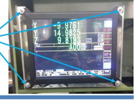
**Step #7)** Use your MK030. Connect your power use MAP307, Plug in power jack into the Monitor. Connect either MAV541 or MAV563 depending on what your Controller uses for suppling video to the Monitor, plug in the 15 Pin side
