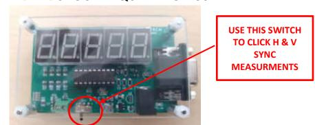
STEP #4) IF YOU ARE NOT GETTING ANY READINGS, OR ODD NUMBER READINGS. YOUR VIDEO CARD IN YOU CONTROLLER IS NOT SUPPLING THE PULSES TO THE ADAPTOR CABLE. OR OUR CABLE HAS THE WRONG PIN OUT.
