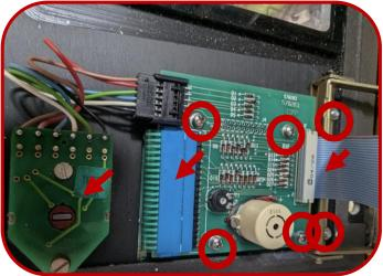
Unplug the video cable from the video card. Remove the video circuit board to give you access to remove the monitor.
